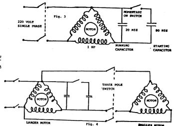
running and 80 microfarads of capacitance per horsepower in parrallel with the 20 microfarads for starting. Since the motor does not have a built-in centrificial switch to switch in and out the starting capacitor, a momentary switch has to be provided for you to switch this capacitance in and out. See Figure 3.
