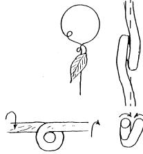
It is best to thin the leaf stem before completely forming the leaf, but don't thin it so much that it breaks or burns off. Work over a rounded edge of your anvil.
