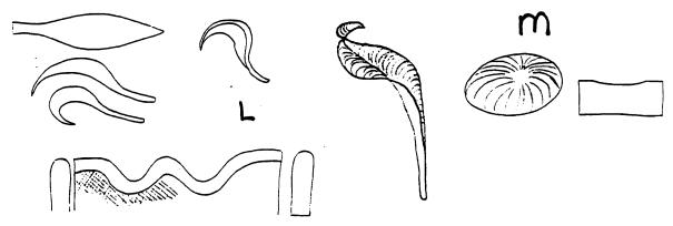
DOUBLE ROUND SHAPE: A bit hard to draw. The design comes to center at a 90°. Start with a flat piece of stock ½" at end, 1" thick in the center and 6" long. (N) Work the 90° right angle on your curved area on your wood block, or serpent stake. I know that it seems nearly impossible, but I called Dick to make sure. He said the metal will move. When finished the object is quite nice. It could be used to suspend a rope for a hanging basket.
