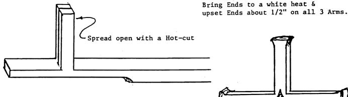
·Hold down with a Hammer on this side to make it stationary.
