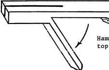
Hammer up this part to top & make flat with Bar.
