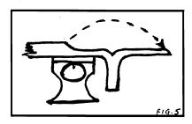
9. UNFOLD THE CUTS TO FORM THE VERTICAL PORTION OF THE CROSS.
