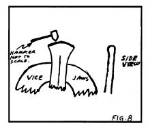
11. UPSET AND ARC THE THREE ENDS OF THE CROSS. FRANCIS STARTS THIS EFFECT WITH A CROSS PEEN AND FIN-ISHES IT WITH THE FLAT FACE OF THE HAMMER.
