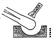
3. Using a hemispheric swage block, dish the head slightly. Form an eye with a round eye punch & add a horizontal pupil slit.
