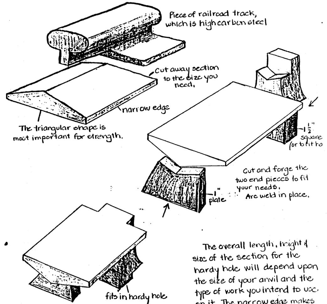
The overall length, height & size of the section for the hardy hole will depend upon the size of your anvil and the type of work you intend to use on it. The narrow edge makes this ideal for smaller intricate pieces of work, such as floral designs.
