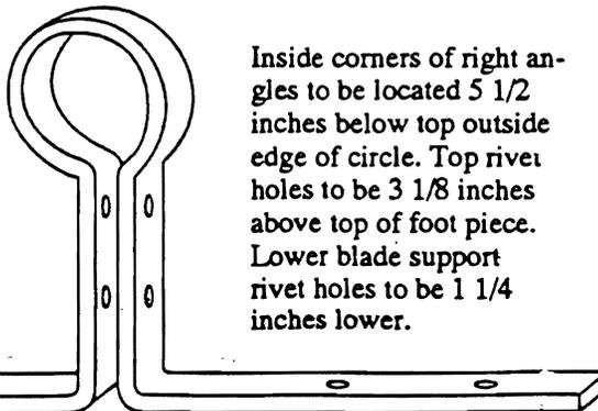
Inside corners of right angles to be located 5 1/2 inches below top outside edge of circle. Top rivet holes to be 3 1/8 inches above top of foot piece. Lower blade support rivet holes to be 1 1/4 inches lower.
