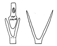
Joe warns not to use a big hammer for fullering job. Use a small hammer, and mak of light blows. Heavy blows will split the area rather create a good Opset.
