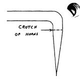
Here is where Joe Anderson's ram's head differs from some other smiths' methods. Some smiths fold the head over on itself and make a weld. Joe doesn't fold the head over, and he doesn't make a weld. Instead, he drives a fuller down herween the horns to upset the head and form a nose.
