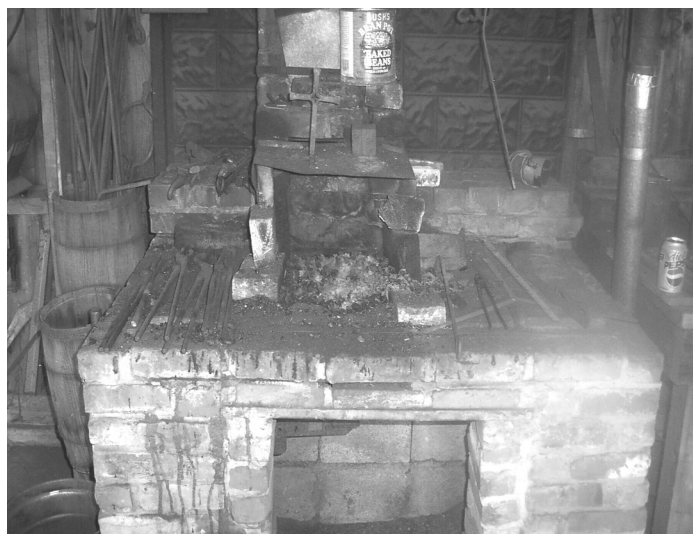
The forge at the Auglaize Village Blacksmith Shop. It is brick with a brick chimney and cast iron firepot
