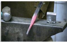
12. Optional step- use hot cut/ hardie tool to fuller small grooves/rings around the snakes tail, if you want a rattlesnake. Beware of cutting off the tail!
