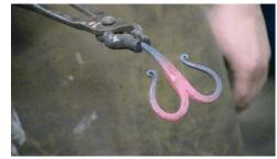
7. The final step was to bend the scrolls back into a graceful hook. He gave the whole buckle a slight bend and bent a small prong on the tapered end.
