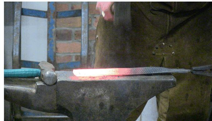
2. At this point, it is a good idea to straighten any bending with a rawhide mallet. Also, it is easy to correct any twisting by any misplaced hammer blows. Make sure to keep it clean with a wire brush as you forge.
