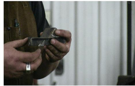
9. Now to the vise! This is a tool Roy uses to aide in punching the eyes and nostrils into the snake. It is called a "v block"- simply put, a triangle piece welded to a scrap piece of angle iron.
