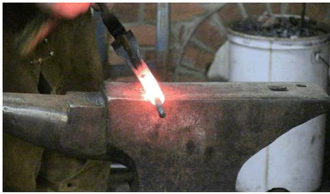
3. Now for the 3/8" bar... put the 3/8" bar in the "u" shape, and close up the tail. Work your way back up to the head of the snake.
