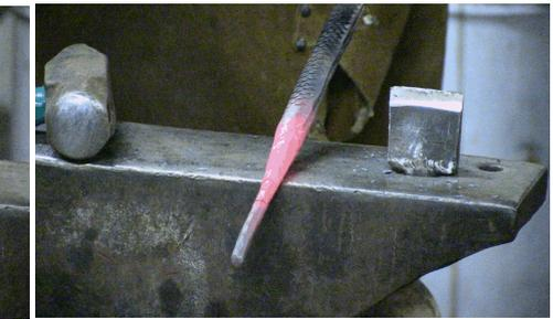
12. Optional step- use hot cut/hardie tool to fuller small grooves/rings around the snakes tail, if you want a rattlesnake. Beware of cutting off the tail!
