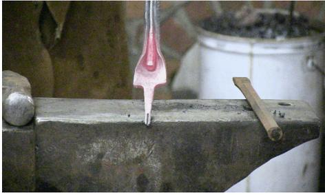
4. Make sure when you put in the bar, it does not come up completely to the tang. Leave this area open for the tongue. At this point, you can start to split the tongue, as pictured.
