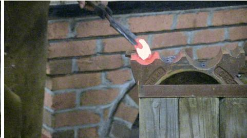
6. Now bend the tongue back into the jaw area, and close up the head and jaw area.
