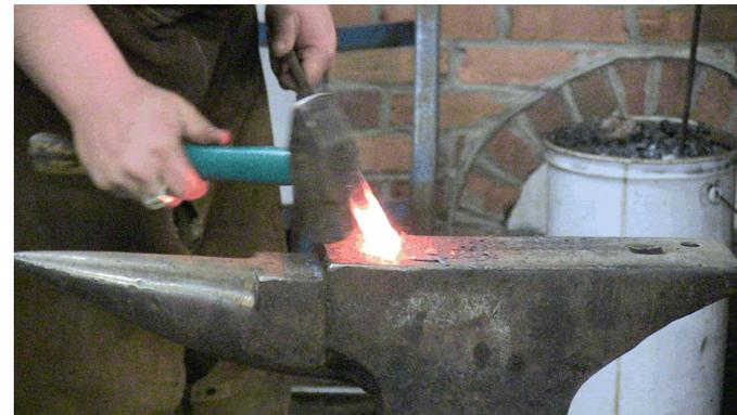
1. You start by rolling up the edges of the rasp using your swage block, being careful not to hammer too hard (that would destroy the scales). You continue doing this for the whole length of the rasp until you get to where the jaws are supposed to be. It should look like a "u".
