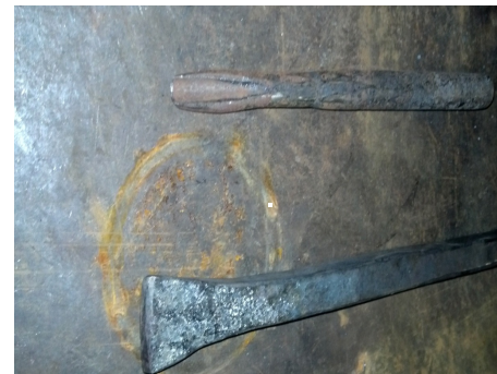
Top: Arc (semi-circular) punch for round eyebrows Bottom: straight punch for incising lines
