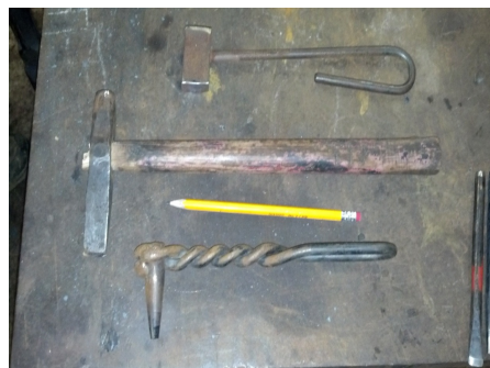
Additional tools that Dick uses for figure work: (From top: set hammer, hot cut, punch.)
