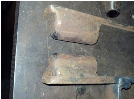
Here is the 3/8 spring swage: (Note how the ends are slightly rounded.)
