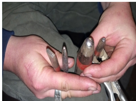
Here are the punches that Dick uses: (From left to right: straight punch for lines, small ball end punch for eye, larger ball end punch for eye, regular eye punch for eye.)
