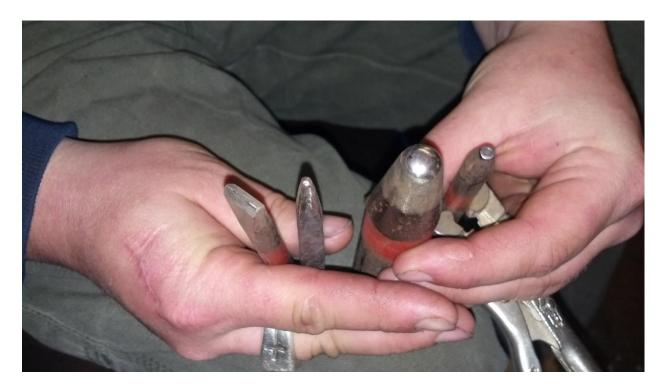
(From left to right: straight punch for lines, small ball end punch for eye, larger ball end punch for eye, regular eye punch for eye.)
