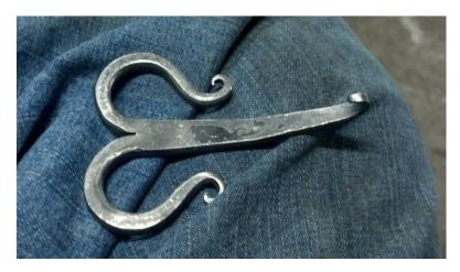
11 – The buckle is now complete but flat. Use a swage block or the widest part of the anvil horn to put a slight curve across the entire length of the buckle. The prong is on the concave side of the curve, the front outside face of the buckle is on the convex side.
