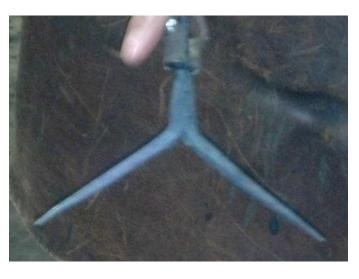
4 – Make a convenience bend to spread the horns out to form a Y shape so you can work them separately. Use the hardy cut to start the split and complete it on the edge of the anvil. The piece will want to distort and fold. Prevent this by returning it flat on the anvil face and straighten it.
